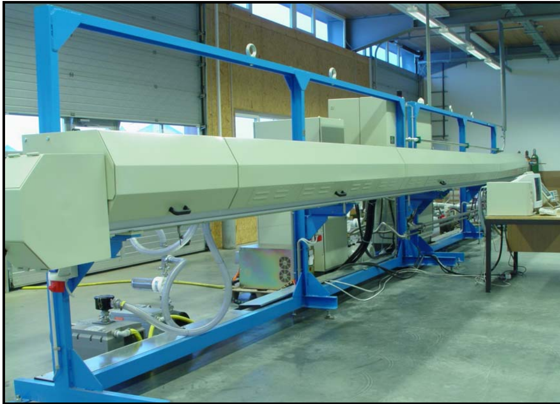
Figure 1. PlasmaANNEALER for high-speed annealing of stainless steel and nickel alloy wires.
